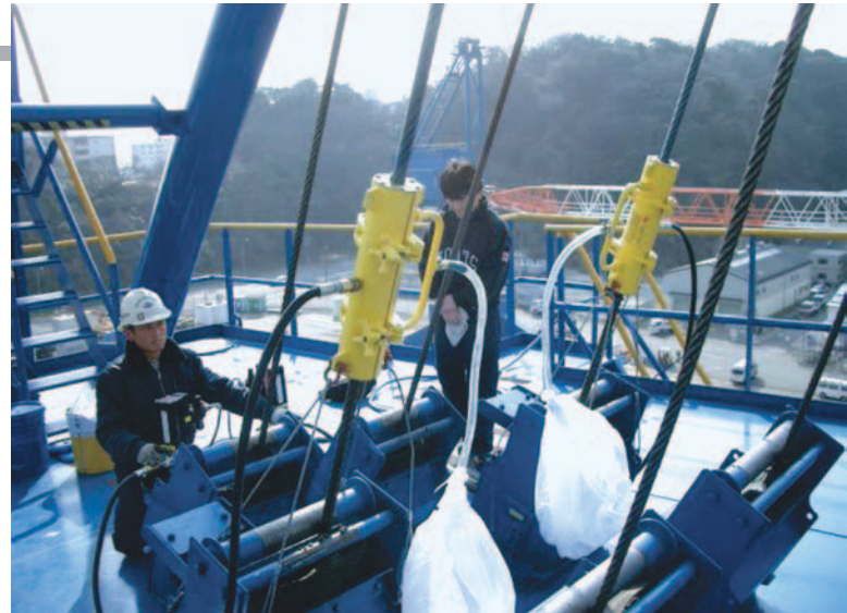
Yokosuka Naval Base Base. Twin SU35B Wire Rope Lubricators used on barge crane.
