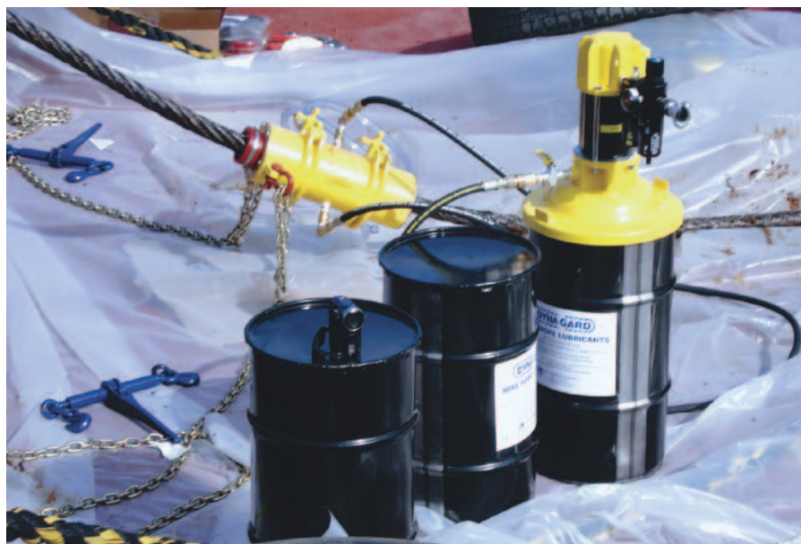
G&H Towing, Galveston Texas USA treating 1,500' of 51mm tow line using Kirkpatrick Model JU120 & Dynagard Blue.
